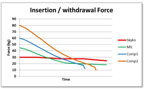
The **Skyko International** 400Hz plug has been designed to have a force of 70 pounds, 30 kg, which is well sufficient to fulfil the two conditions of electrical contact and holding into position.
